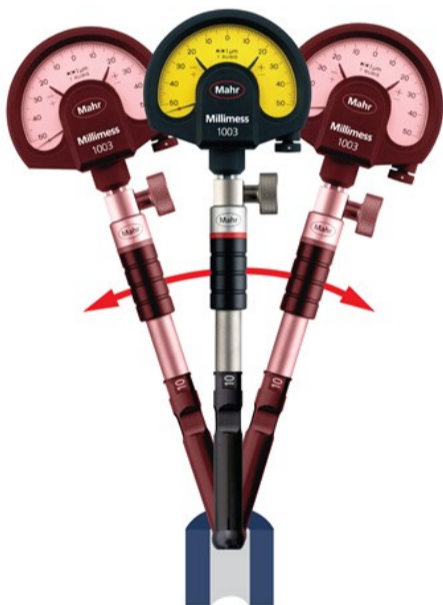
Left-right rocking of gage in bore. Photo Credit: Mahr Inc.
