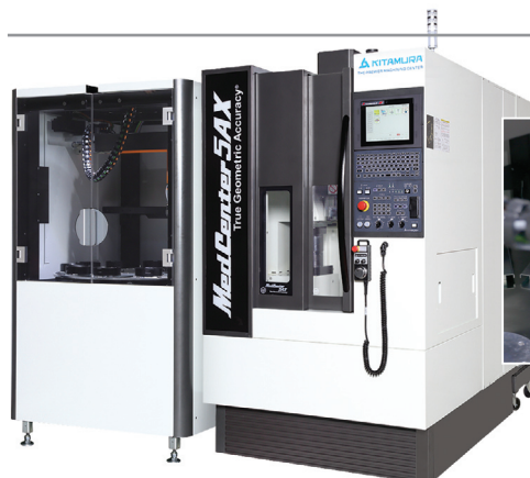
12 Pallet APC System with 280 x 280mm (11" x 11") pallet tables.
