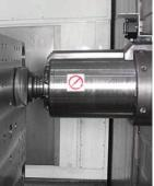
With Power to handle the toughest cutting conditions the Mycenter-HX8000G/1000 features a 53HP. high-torque, 4-step gear driven spindle that delivers high-efficiency cutting performance with low energy consumption. 8,000min<sup>-1</sup> and 12,000min<sup>-1</sup> configurations are available.
