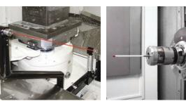
Spindle and Tool Probes
