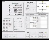
Work Set Assistance. Set-up work offsets with just a few keystrokes. Four types of measurements are possible. Edge side measure, center measure, 3 point diameter center measure and corner measure if
