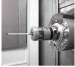
Spindle and Tool Probes
