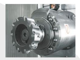
driven spindle that delivers high-efficiency cutting performance with low energy consumption, 8.000min<sup>-1</sup> and 12.000min<sup>-1</sup> configurations are available.
