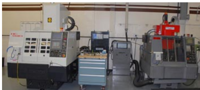
CM&D's side-by-side Roku-Rokus are ten years apart in age. The new HC-548EX hybrid satisfies the company's needs for steel and graphite.
